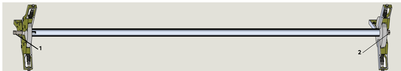
Fig. 16.2.2 RS6054-001, 3 wing steel shaft assembly
